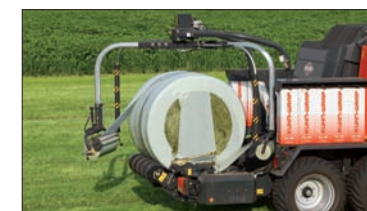
3D wrapping distributes film more uniformly and efficiently across the entire surface of the bale (VBP only)
