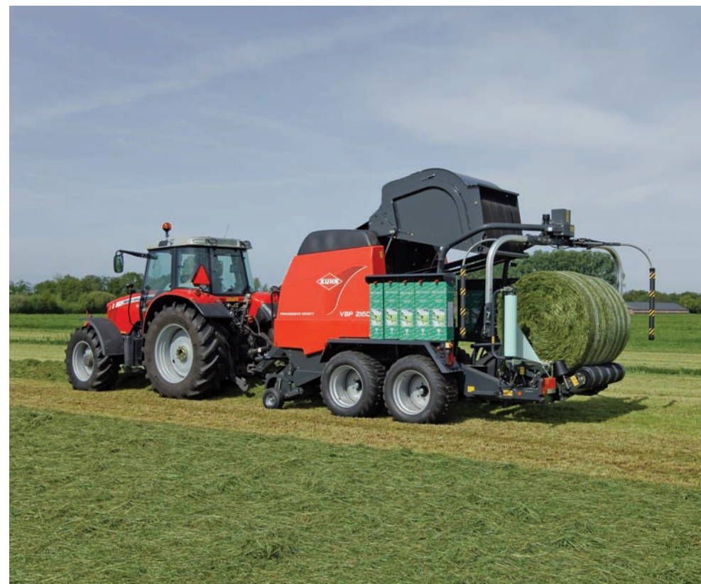
The bale is covered with 3 layers and 67% overlap
