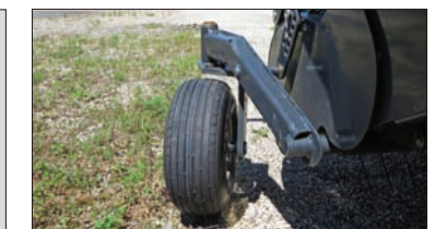
Pivoting pickup wheels for extreme conditions to ease wheel and tire stress
