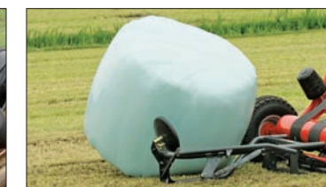
Bale turner gently places the bale on a flat end during unloading (VBP only)
