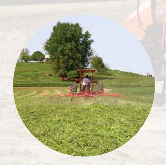
Rotary tedder with four rotors, 17'1" working width and hydraulic folding.
