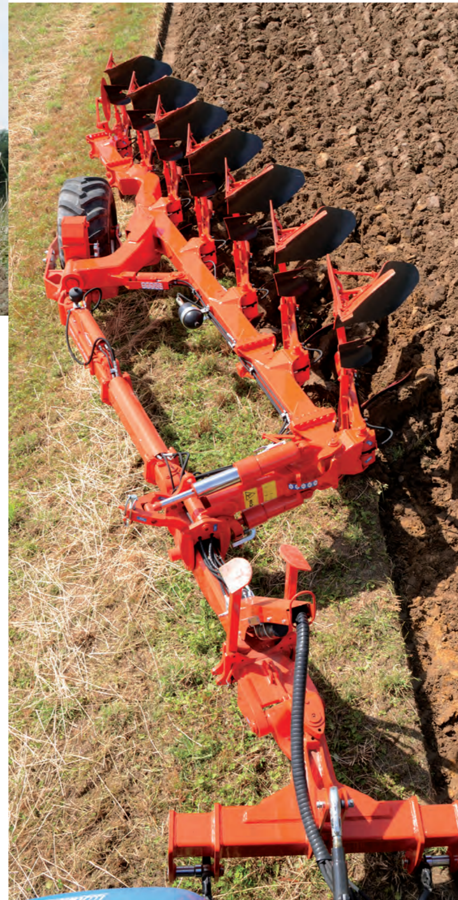
Hydraulic sequencing comes standard meaning fewer valves to operate during headland turns.
